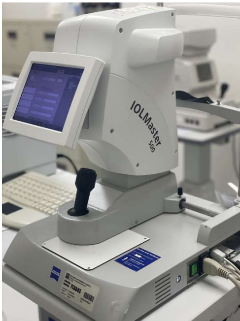
Fig. (2). IOLMaster by Carl Zeiss Meditec—an advanced device used for precise measurements of the eye's axial length, corneal curvature, and anterior chamber depth.
