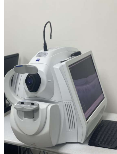
Fig. (3). Optical Coherence Tomography (OCT) machine by Carl Zeiss Meditec, Dublin—used for high-resolution imaging of retinal structures.
